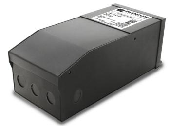
Magnitude's T300L12DC is a multi-output class 2 LED dimmable LED driver. It is equipped with push-to-reset breakers, one on each output, protecting both the load and the driver. Encased in a high-quality NEMA 3R metal case enclosure, that includes 5 knock-outs to enable easy installation. All of our T- Series LED Drivers are dimmable with any standard MLV TRIAC dimmer.
