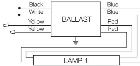
Note: For one lamp application, cap two yellow leads. Insulate to 600 volts.
