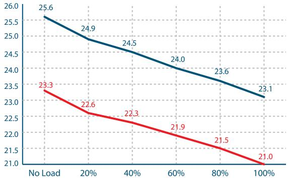
Output Voltage vs. LoadOutput Voltage With a Typical Dimmer
