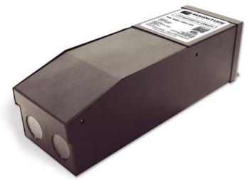
Magnitude's M150L24DC-AR is the most compact LED driver on the market with a magnetic transformer core. It is equipped with two auto-reset breakers, one on the input and one on the output, which protect both the load and driver. The driver is encased in a coated metal box that includes 4 knock-outs, to enable easy installation that complies with electrical code requirements.
