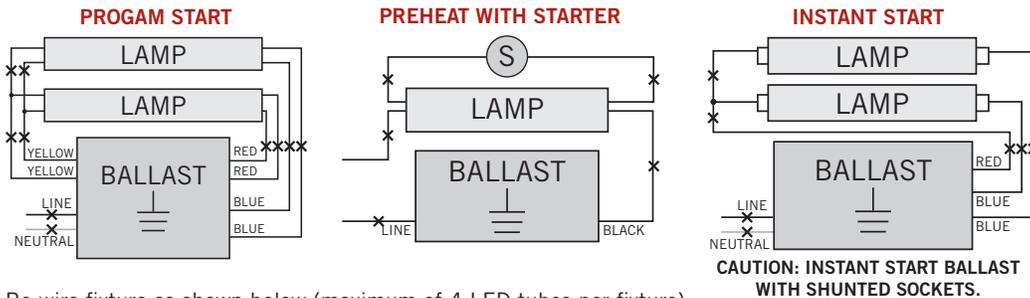
Re-wire fixture as shown below (maximum of 4 LED tubes per fixture).
