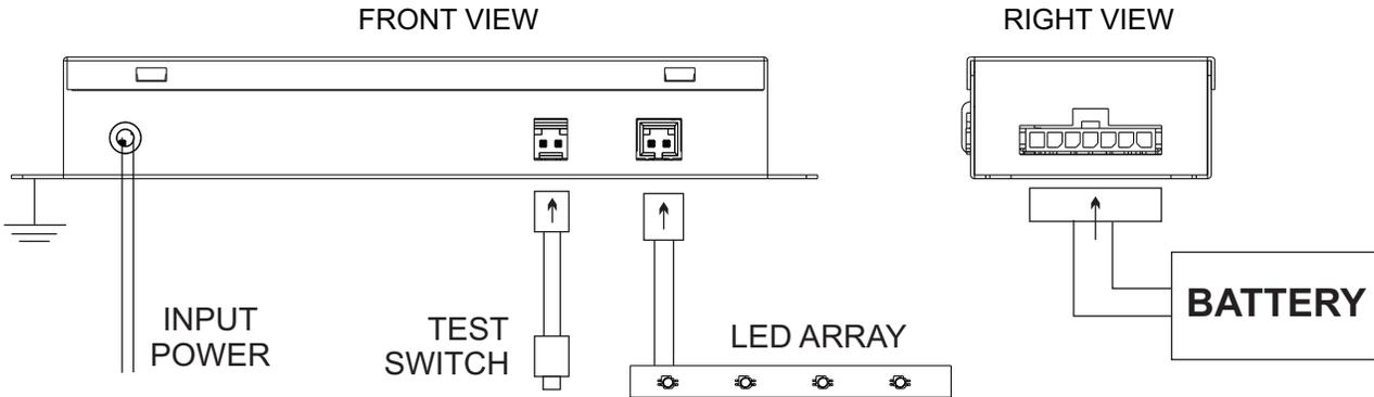
**IMPORTANT:** Do not connect battery until fixture is installed
