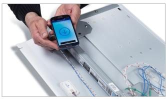
Step 1: Place the smartphone next to the NFC antenna on the driver.
