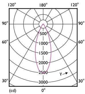
LEDspots N DIM 13W PAR38 E26 930 40D-LDD
