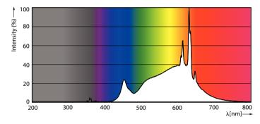
Spectral Power Distribution Colour - 10PAR38/LED/930/F40/DIM/ GULW/T20 6/1FB
